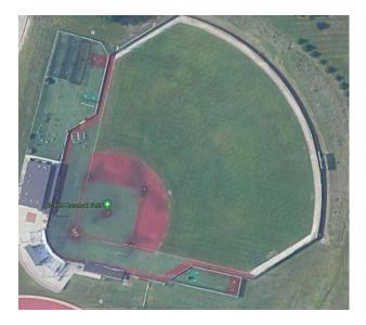
**Optional Bid Addition #2 – 3ft Turf Transition Strip Along Left/Right Foul Lines.** Install 3 ft strip of turf adjacent to left and right foul lines to the new turf infield to provide separation from grass. Either a nailing board or concrete curb is acceptable to hold the transition strip in place. Color to be selected by owner (Note blue lines are what is covered in this Option)
